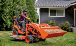
**BX2380RV60-1** w/ LA344S & 60" Mower • 21.6 Gross HP,<sup>†</sup> 3-Cyl. Kubota Diesel Engine • 4WD • Category I, 3-Point Hitch
