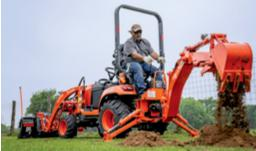
BX23SLSB-R-1 w/ BT2416 16" Backhoe Bucket • 21.6 Gross HP,<sup>+</sup> 3-Cyl. Kubota Diesel Engine
